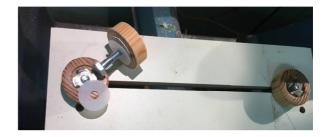
I cut some 30 x 30mm squares, made an MDF/plastic sandwich using masking tape to hold it together and drilled a 6.25mm hole in the centre.
